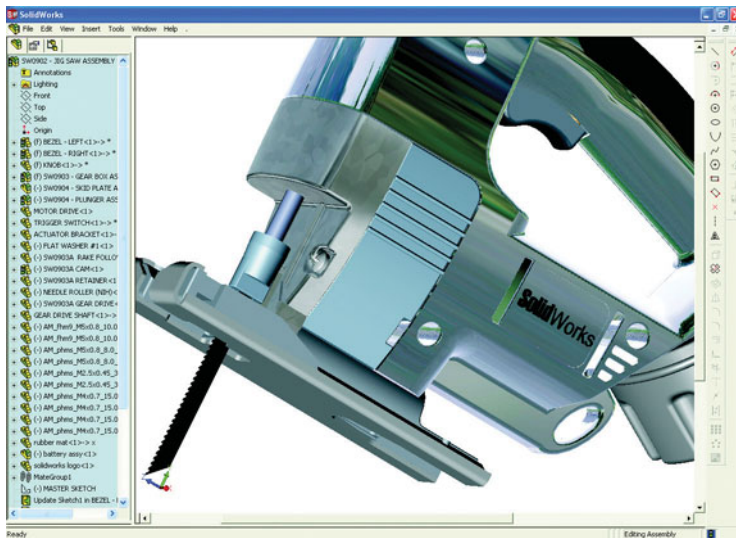
Color Plate 1 Screen shot of the SolidWorks application, showing a jigsaw rendered with OpenGL shaders to simulate a chrome body, galvanized steel housing, and cast iron blade. (Courtesy of SolidWorks Corporation)
