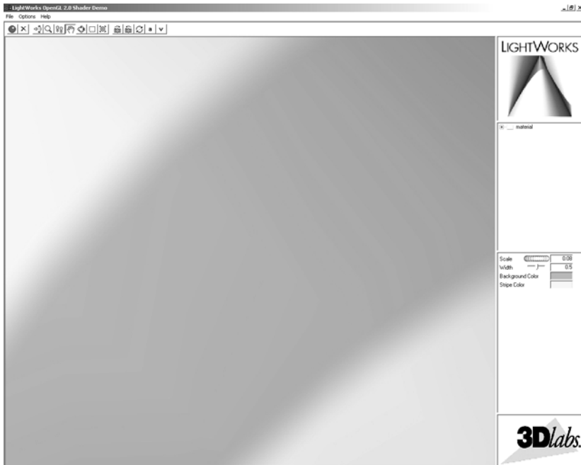
Figure 11.2 Extreme close-up view of one of the stripes that shows the effect of the “fuzz” calculation from the stripe shader (courtesy of LightWork Design)
