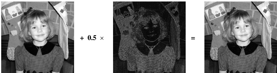
Figure 19.3 Results of the unsharp masking shader. (Laplacian image in center is scaled for display.) Zoomed views of the original and resulting images are shown in Figure 19.4.
