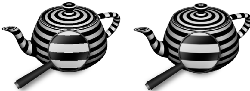
Figure 17.6 Effect of adaptive analytical antialiasing on striped teapots. On the left, the teapot is drawn with no antialiasing. On the right, the adaptive antialiasing shader is used. A small portion of the striped surface is magnified 200 percent to make it easier to see the difference.
