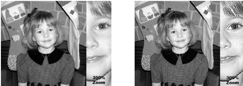
Figure 19.4 Results of the unsharp masking shader. Original image is on the left, sharpened image on the right.
