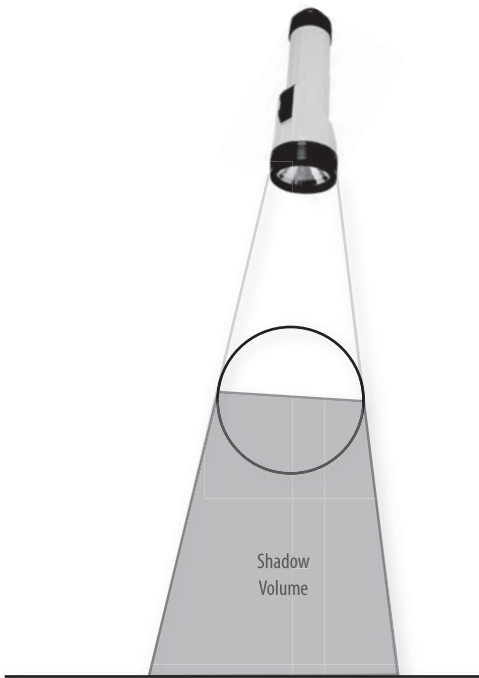
Figure 13.2 The shadow volume for a sphere
