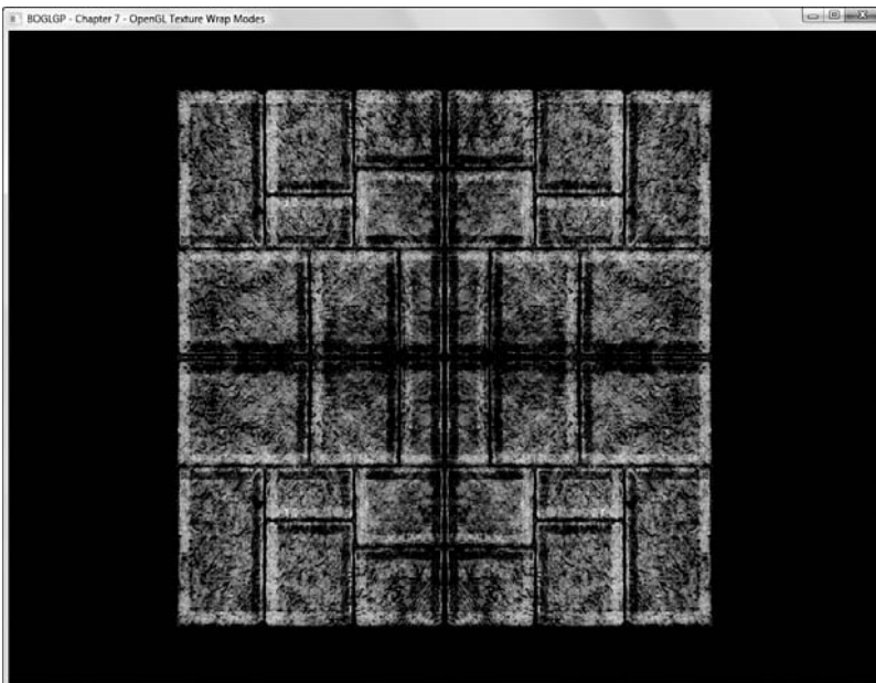
Figure 7.6 Wrap mode GL_MIRRORED_REPEAT .
