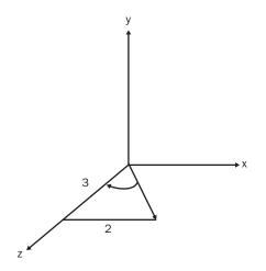
The second rotation about the x-axis rotates the eye vector into the yz plane, which will leave the eye vector pointing in the direction of +z. The angle of rotation can be calculated by projecting the eye vector into the yz plane, like this:
