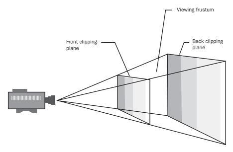
You can either build a matrix or use the *D3DXMatrixPerspectivexxx* helper functions.
