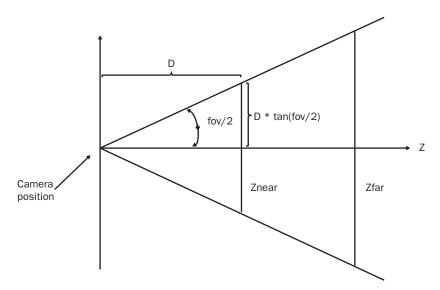
This figure shows the front clip plane,  $Z_{NEAR}$ , and the back clip plane,  $Z_{FAR}$ . This figure is a side view of the viewing frustum, where *fov/2* represents the vertical field of view angle. D represents the distance between the camera and the near clip plane.
