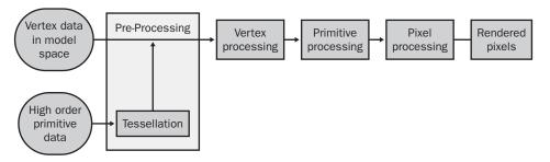
Vertex processing converts per-vertex data from model space to projection space. This appendix goes into more detail about the major vertex processing blocks, including transformations, vertex fog, and per-vertex lighting and material colors.
