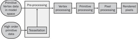
As we saw in Chapter 1, the pipeline processes per-vertex data to convert geometry from model space to projection space. After vertex processing, primitive processing and pixel processing convert per-vertex data into the final pixels that will be rendered.
