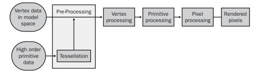
Vertex shaders are executable programs that process vertex data. In the fixed function pipeline, Vertex processing takes primitive vertex data from model space and converts it into vertex data in projection space. Before we go any further, let's define some of the terms we just used.
