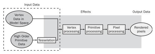
The pipeline transforms input data into output pixels that fill the frame buffer. The input data comes from objects that are made up of vertices in model space or higher-order surfaces created from N-patches, rectangle patches, and triangle patches. Once the input data has been tessellated, the pipeline performs vertex processing, primitive processing, and pixel processing before outputting the final pixel colors.
