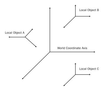
A world transform can consist of a translation, a rotation about any of the axes, and a scale along any of the axes, which would be represented by this equation:
