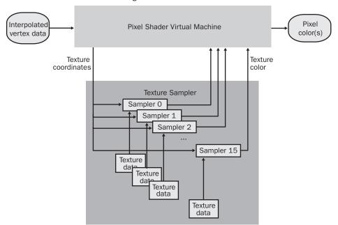
Pixel Processing Part 1 (detailed) Programmable Pixel Shader
