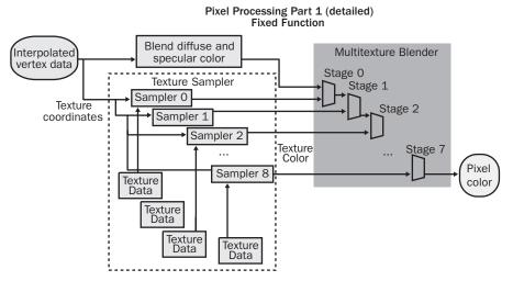
The texture sampler is made up of texture data and samplers.
