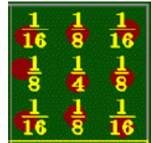
Down-sampled with a 5x5 Gaussian filter (non-uniform weights)
