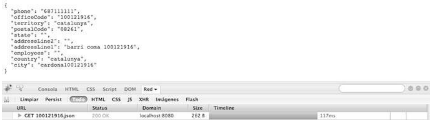
Fig. 15.6 A JSON representation processing time for the /office/100121916 resource
