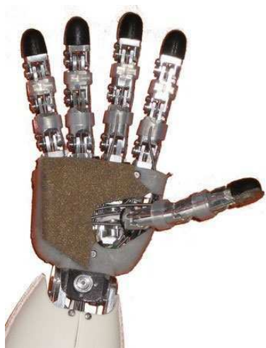
Fig. 7.2 The iCub hand has three independent fingers (including the thumb) while the fourth and fifth fingers are used for additional stability and support and have one DOF overall
