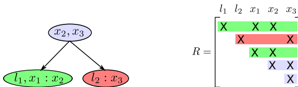
Fig. 2 The Bayes tree and the associated square root information matrix R describing the clique structure in the Bayes net from Fig. 1. A Bayes tree is similar to a clique tree, but is better at capturing the formal equivalence between sparse linear algebra and inference in graphical models. The association of cliques with rows in the R factor is indicated by color.
