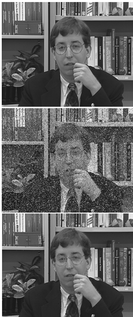
Fig. 5 20-th frame of the “Deadline” video sequence: top = original frame, middle = noisy frame (25% random impulse noise), bottom = result of our FRINV-G filter.
