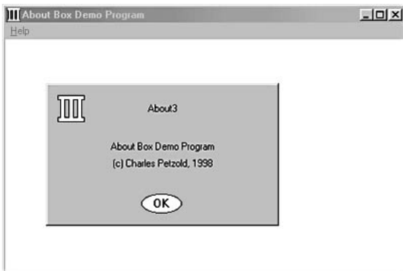
Figure 11-6. A customized push button created by ABOUT3.
