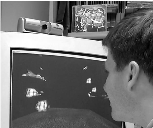
**Figure 14** A computer monitor with a video camera can be a very simple VR display, referred to as “fishtank VR” due to the similarity with looking into an aquarium. (Copyright 2003, William Sherman.)
