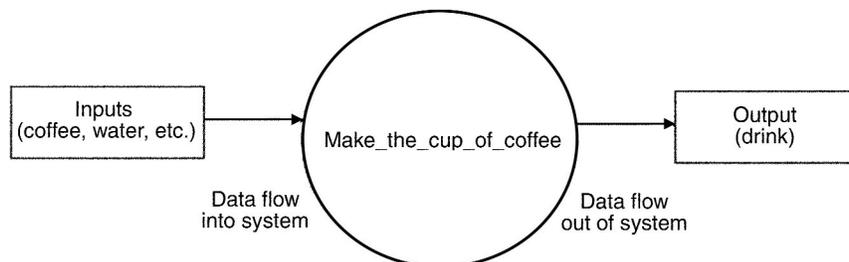
**Figure 2** Data flow diagram for a coffee making example.
