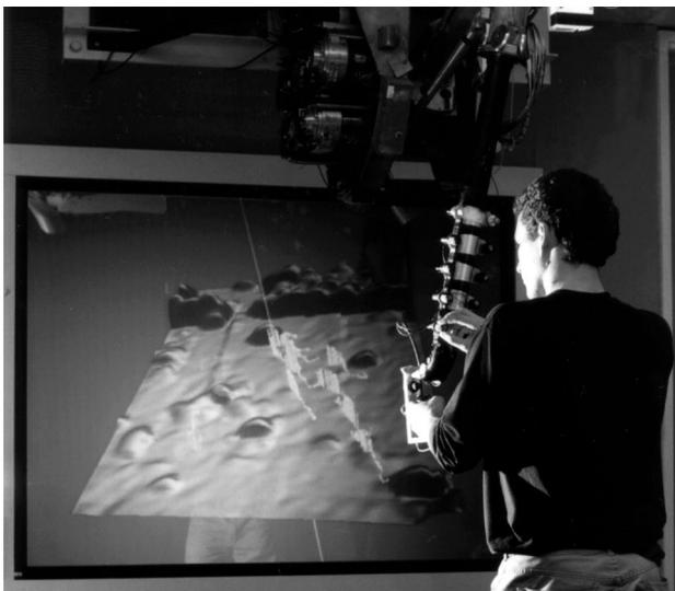
**Figure 15** This world-grounded haptic force-feedback device is attached to the ceiling, allowing a user to grab the controls and interact with the molecular world. (Image copyright 1994, the University of North Carolina at Chapel Hill.)
