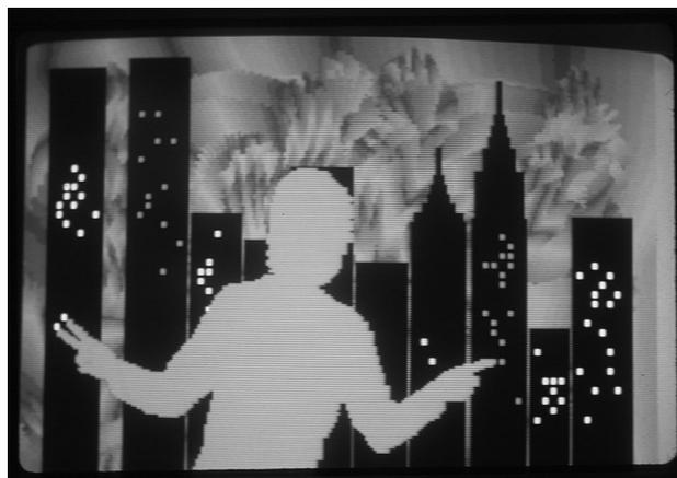
**Figure 3** In Krueger's *artificial reality*, a video camera is used to place an overlay of the participant's body on the virtual world. (Image courtesy Myron Krueger.)
