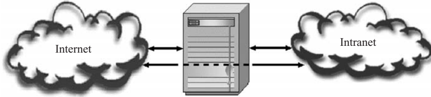
Figure 4: Dual-homed proxy with IP forwarding.
