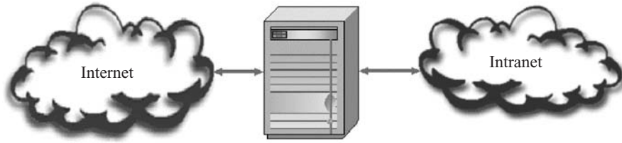
Figure 3: Dual-homed proxy without IP forwarding.
