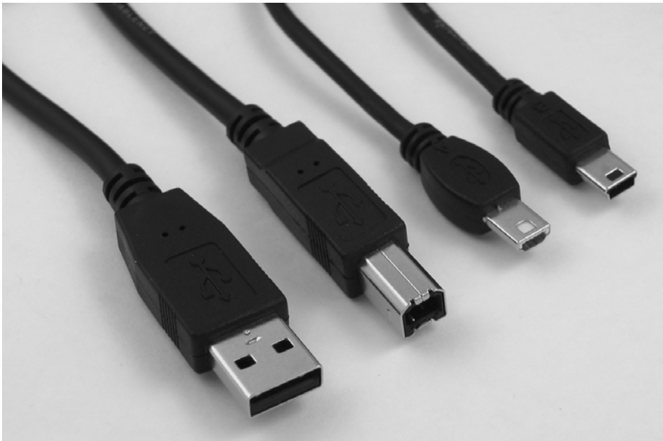
Figure 19-7: The USB specifications define four plug types. From left to right, they are Series A, Series B, mini-A, and mini-B.
