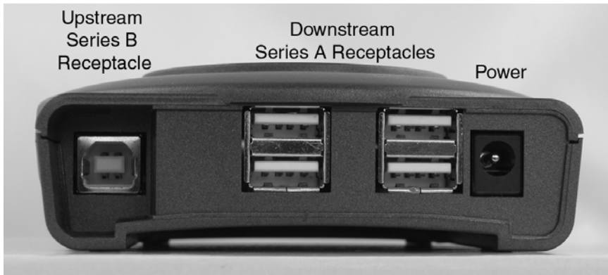
Figure 15-1: A hub has one upstream port and one or more downstream ports.
