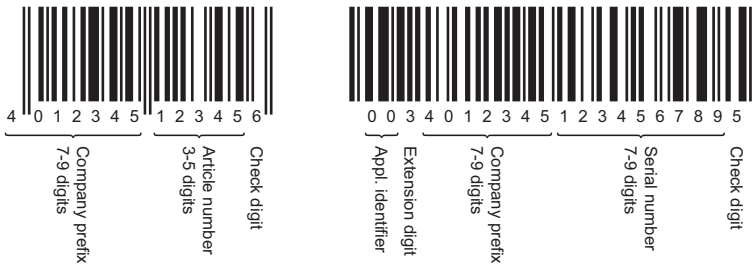
Fig. 3.5 EAN-13 (left) and SSCC (right) are intended to encode article numbers and numbers of shipping units, respectively. Both of them contain started by the GLN company prefix of their company. The application identifier 00 is part of the EAN128 bar code encoding standard for SSCC.
