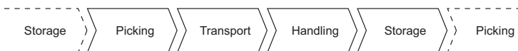
Fig. 7.6 The primary logistics functions of storage and transport alternate. Two storage locations can be connected by one transport operation. Between each pair of storage and transport operators, it is necessary to apply handling and picking operators, respectively.
