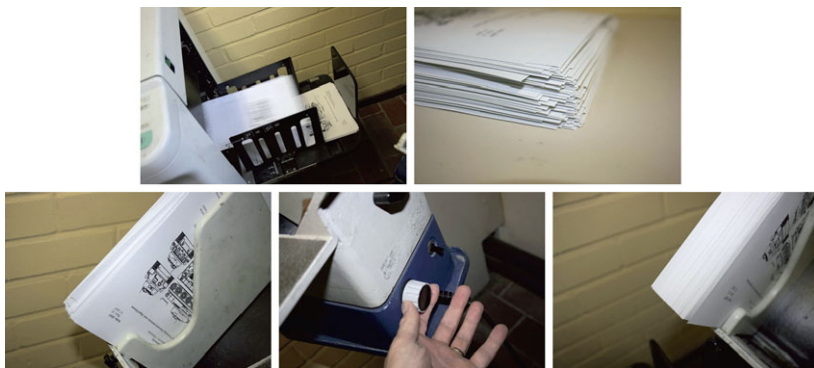
Fig. 41.5. The exercise sheets come out of the printing machine. The edges are not aligned. The paper jogger shakes them, and in the end we get a perfectly aligned stack of paper
