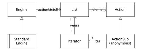
The object model shows how an action belonging to an action list of an engine has access to that list indirectly via an iterator.
