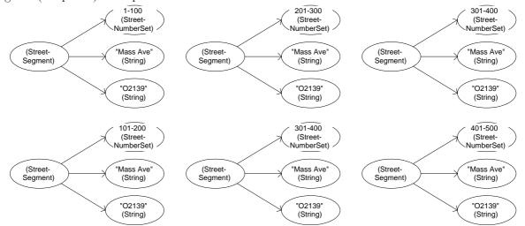
This representation is correct (for instance, all pairs of street names return true when compared with equals), but it is unnecessarily wasteful of space. This would be a better runtime configuration of the system:
