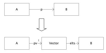
In our Folio Tracker example, we might replace interpose a vector in the relation *posns* between *Folio* and *Pos*. Note the mutability markings; the collection is usually constructed and garbage collected with its container.
