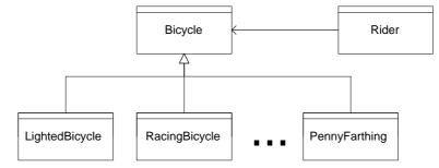
Even though there are just as many arrows, this diagram is much simpler than the original one: dependence edges complicate designs and implementations more than other types of edge.
