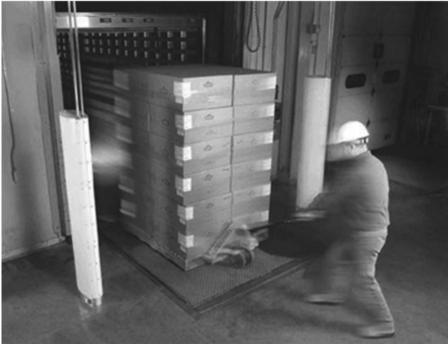
FIG. 12. Typical RFID-enabled warehouse loading bay portal.
