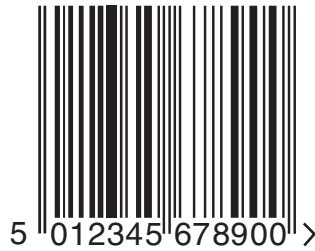
FIG. 2. A typical example of an EAN-13 bar code.
