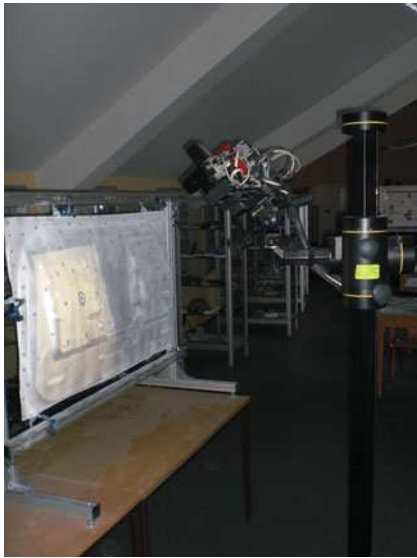
Fig. 2 Vertical clamping frame with die formed part and 3D-Scanner ATOS
