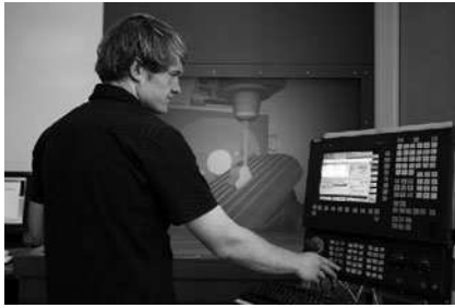
Fig. 4 HiL coupling between Siemens SINUMERIK 840Di and a virtual machine model
