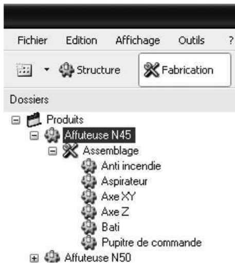
Fig. 10 Manufacturing decomposition of a grinding machine
