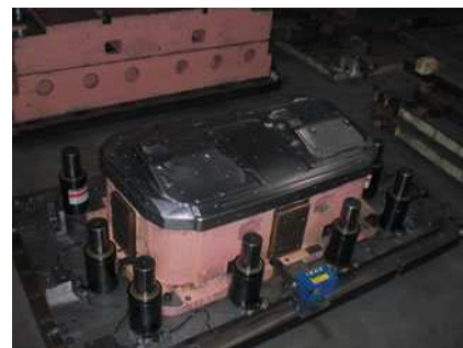
Fig. 3 Incorporated die (ram) with reference points for photogrammetry and 3D scanning
