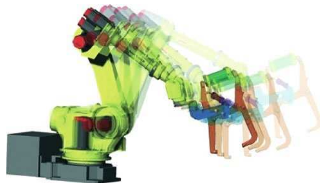
Fig. 2 Kinematic analysis of a welding robot [1]
