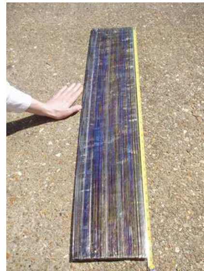
Fig. 3 1000 mm × 200 mm × 4 mm RUAM titanium wall structure
