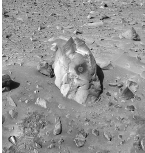
This image of the Martian rock “Humphrey” shows a hole made by a grinding tool carried on the Mars Exploration Rover Spirit , which landed on Mars on January 4, 2004. The grinding process revealed the inner structure of the rock and produced a sample that could be tested for chemical composition. (NASA/JPL/Photo Researchers, Inc.)
