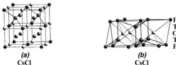
Figure B.9. (a) Eight CsCl cells, \text{Cs}^+ ions are in the centers of cells (T sites). \text{Cl}^- ions, at the corners, are in P sites (dark spheres) and O sites (light spheres). (b) A side view showing the spacings of the layers.
