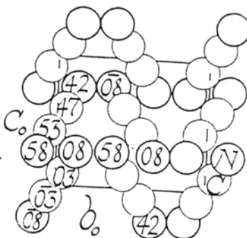
Figure 11.4. The face-centered orthorhombic crystal structure of cyanogen. The structure projected along the a_0 axis. Heights along a_0 are shown.
