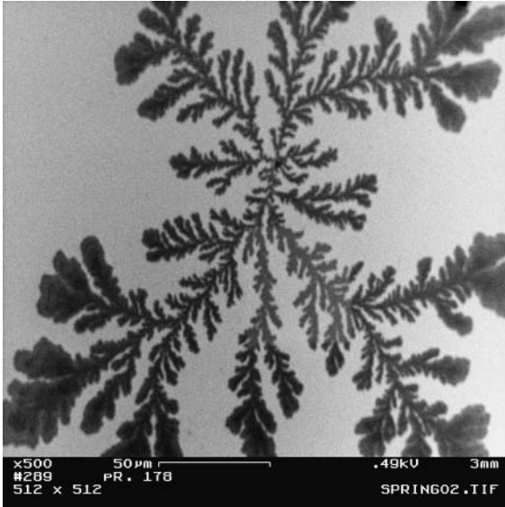
Fig. 8 Increase of tip-radii and multilamellae at the end of the dendrite due to changing of diffusion conditions during isothermal crystallization at limited material supply.
