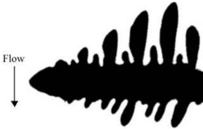
Fig. 5 Phase-field simulation of dendritic growth in a flow, showing that the predominant morphological effect is an asymmetry in the side-branch structure, with side arms growing preferentially into the flow.
