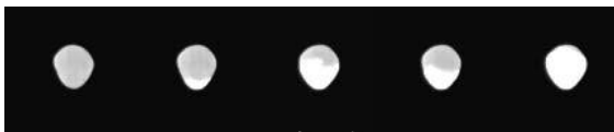
Fig. 9 Solidification of silicon undercooled at 255 K recorded with the high speed camera
