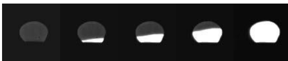
Fig. 10 Solidification of silicon undercooled at 330 K recorded with the high speed camera
