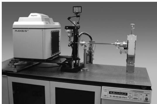
**Figure 5.1** Raxis IV<sup>++</sup> mounted on a generator. The rotating anode wheel is on the far right and the long optics is clearly visible. The detector is on the left and in front of this is an inverted  $\varphi$ -axis. (Courtesy of Dr Joseph Ferrara, Rigaku Americas Corporation.)
