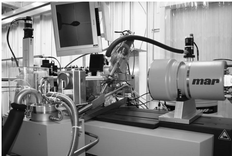
**Figure 12.2** SGX-CAT data acquisition station. The CCD detector and cryogenic sample handling robot appear in the foreground. The pump to deliver the liquid nitrogen that removes ice from the sample is located at the rear right.
