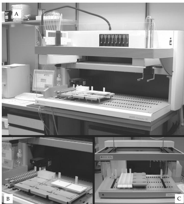
**Figure 14.3** The Genesis workstation from Tecan. (a) A general view of the workstation. The two mobile arms move above the deck supporting the microplates. (b) A close-up view of the deck supporting the microplates. (c) The Miniprep 75 workstation is very handy when one needs to prepare crystal screening solutions from mother solutions.
