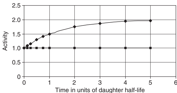
FIGURE 9.2 Activity of a sample exhibiting secular equilibrium. The timescale is in units of half-life of the daughter and activity is in arbitrary units. Note how the total activity approaches a value that is twice that of the parent at longer times.
