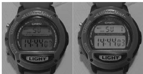
Figure 2-1. The application of electroluminescence in lighting the display in this watch. An electric signal, caused by pressing the “light” button on the watch, excites the molecules in the display medium that cause luminescence upon their relaxation (see color plate section)
