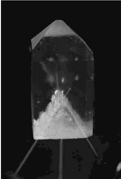
Figure 2-2. A non-linear optical material, ammonium dihydrogen phosphate, displaying second-harmonic generation, the frequency doubling of light (infrared to blue). The origin of this physical phenomenon is entirely dependent on ionic displacement or molecular charge-transfer (see color plate section)
