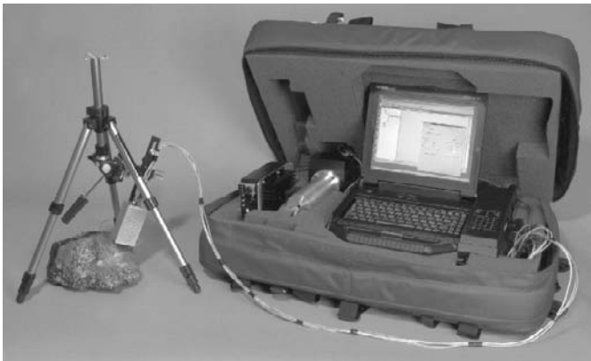
Figure 1-18. Miniaturised Raman spectrometer prototype for space mission, mass 1 kg
