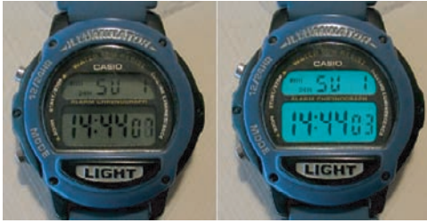
Figure 2-1. The application of electroluminescence in lighting the display in this watch. An electric signal, caused by pressing the “light” button on the watch, excites the molecules in the display medium that cause luminescence upon their relaxation
