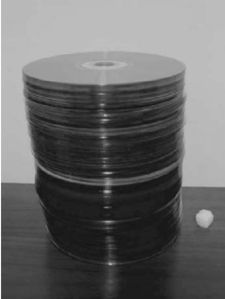
Figure 2-3. A photograph of 100 stacked DVD and a sugar cube. If holographic storage achieves its expectation, one will be able to store a terabyte (1000 Gb) of data in a crystal of size a sugar cube. Employing current commercial optical storage devices, a terabyte of data would fill more than 1000 compact disks, or over a 100 DVD. The use of a sugar cube as a placebo here is a deliberate attempt to emphasise the fact that, although optical technology is developing rapidly, scientists are still struggling to find suitable materials for the application
