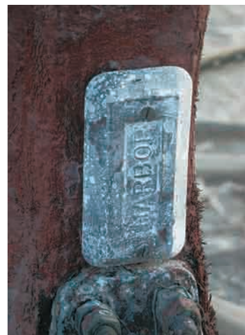
Figure 11.29 Magnesium, zinc, or aluminum blocks are attached to ships' hulls, oil and gas pipelines, underground iron pipes, and gasoline storage tanks. These reactive metals provide cathodic protection by acting as a sacrificial anode.
