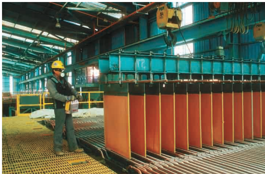
Figure 11.25 This electrolytic cell is used to refine copper. The anode is impure copper, and the cathode is pure copper. During electrolysis, the impure copper anode dissolves, and pure copper is plated onto the cathode. The resulting cathode is 99.99% pure metal. Most impurities that were present in the anode either remain in solution or fall to the bottom of the cell as a sludge.
