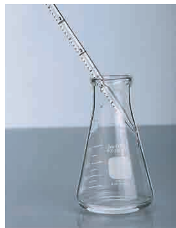
Figure F.3 You can prevent a “stubborn” drop from clinging to the pipette tip by touching the tip to the inside of the glass surface.
