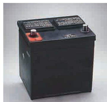
Figure 11.18 A typical car battery consists of six 2-V cells. The cells are connected in series to give a total potential of 12 V.
