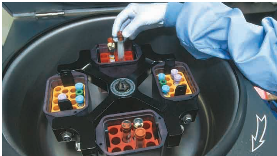
Figure 9.8 Chemists use a centrifuge to separate a precipitate from a solution. The centrifuge spins the samples quickly, and the resulting force pushes the precipitate to the bottom of the test tube. The solution can then be decanted.
