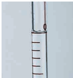
Figure F.2 The bottom of the meniscus must align exactly with the etched mark.
