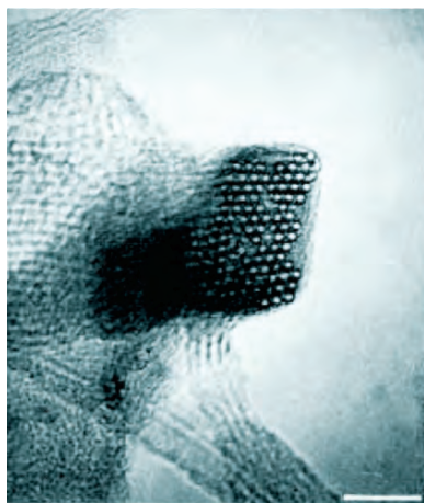
Figure 6.52. High-resolution TEM image of a bundle/rope of single-wall carbon nanotubes, formed spontaneously through the self-assembly of individual SWNTs (scale bar is 10 nm). Reproduced with permission from Thess, A.; Lee, R.; Nikolaev, P.; Dai, H.; Petit, P.; Robert, J.; Xu, C.; Lee, Y. H.; Kim, S. G.; Rinzler, A. G.; Colbert, D. T.; Scuseria, G. E.; Tomanek, D.; Fischer, J. E.; Smalley, R. E. Science 1996 , 273, 483. Copyright 1996 AAAS.
