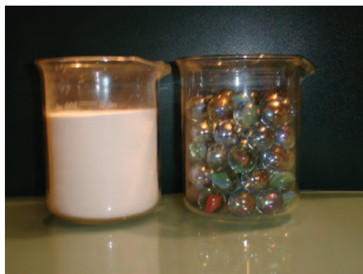
Figure 6.4. Comparison of the surface area/volume ratio of macroscopic particles (marbles) and nanoscopic aluminum oxide particles. Since nanoparticles contain a proportionately large number of surface atoms, there are a significantly greater number of adsorption/reaction sites that are available to interact with the surrounding environment. Further, whereas bending of a bulk metal occurs via movement of grains in the > 100 nm size regime, metallic nanostructures will have extreme hardness, with significantly different malleability/ductility relative to the bulk material.
