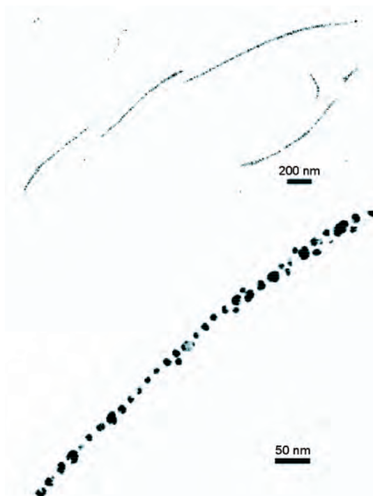
Figure 6.43. TEM images of a 1D array of Au nanoparticles formed through the interaction of PEO and polysaccharide chains. Reproduced with permission from Takagi, K.; Ishiwatari, T. Chem. Lett. 2002 , 990. Copyright 2002 Chemical Society of Japan.
