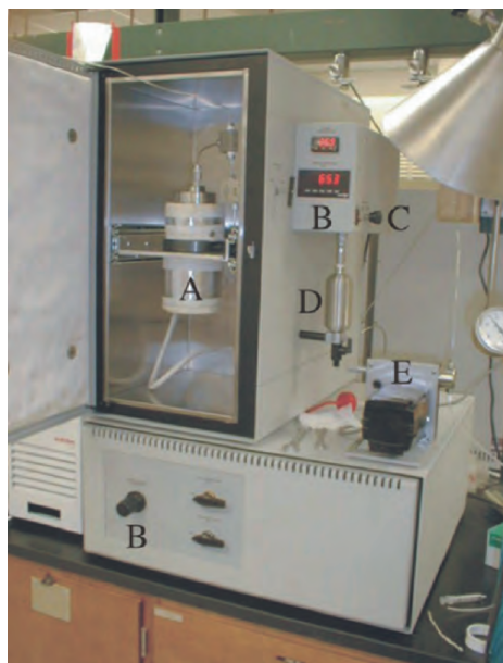
Figure C.2. Photograph of the supercritical fluid system used for nanoparticle synthesis. Shown is the 300-mL high-pressure reactor (A), with pressure/temperature controllers (B). The system is rated for safe operation at temperatures and pressures below 200°C and 10,000 psi, respectively. The vessel may be slowly vented, or exposed to a dynamic CO 2 flow, using a multistage restrictor valve (C), which provides a sensitive control over system depressurization, allowing for the collection of CO 2 -solvated species in the stainless steel collector (D). For deposition using the rapid expansion of the supercritical solution (RESS), nanoparticles were blown onto a TEM grid that was placed under the stopcock below D. Also shown is the cosolvent addition pump (E) used for the synthesis of aluminum oxide nanoparticles, capable of delivering liquids into the chamber against a back-pressure of \leq 5,000 psi.
