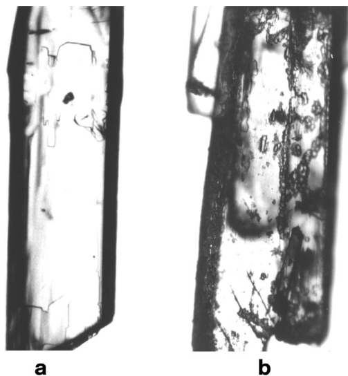
Figure 2.1.4 Micrographs of \alpha -cinnamic acid 1 crystals from benzene on (010) (200-fold in the microscope): (a) fully transparent after 6 months storage under argon in the dark; (b) same crop crystal that turned dull after 6 months exposure to filtered daylight under argon, exhibiting cracks along the (10–1) cleavage plane direction, crystallites on (010), and particularly crystallites on the side faces.
