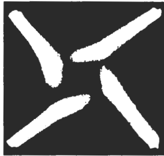
Plate 5.1: Direct flame photograph ( A/F = 17 , \theta = 6^\circ ) [932].
