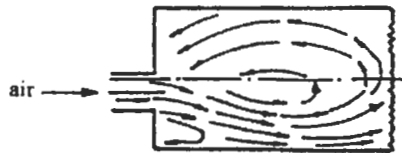
Fig. 4.19(a): Schematic diagram of an asymmetric jet air [603]. Reproduced by permission of ASME.
