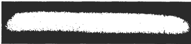
Plate 2.1: Direct flame photograph for methane-air flame at \phi = 1 , 0.1 atm and 300 K.
