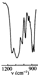
Figure 3.72 IR spectra of [\text{Pt}(\text{DMSO})_4](\text{ClO}_4)_2 in the \nu(\text{S}-\text{O}) region (the broad band at 1100\text{ cm}^{-1} is owing to the perchlorate group). (Reprinted with permission from Inorg. Chem. , 1972, 11 , 1280. Copyright (1972) American Chemical Society.)
