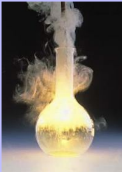
Sodium and chlorine react rapidly to form sodium chloride, the white cloud rising from the flask.
