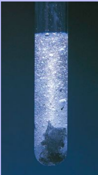
Zinc metal reacts with aqueous acids to produce hydrogen gas and \text{Zn}^{2+} ions.
