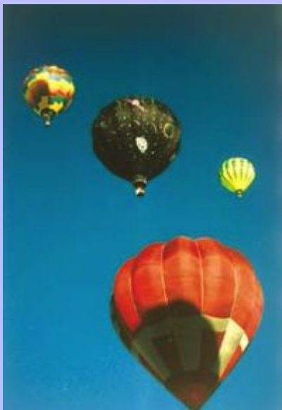
Hot-air balloons rise because hot air is less dense than cooler air.
