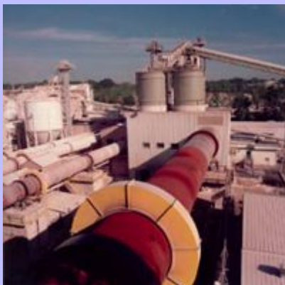
Modern limestone kilns use blowers as well as vents and are computer-controlled.
