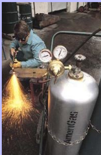
Acetylene is a high-energy molecule used as a fuel for oxyacetylene welding.
