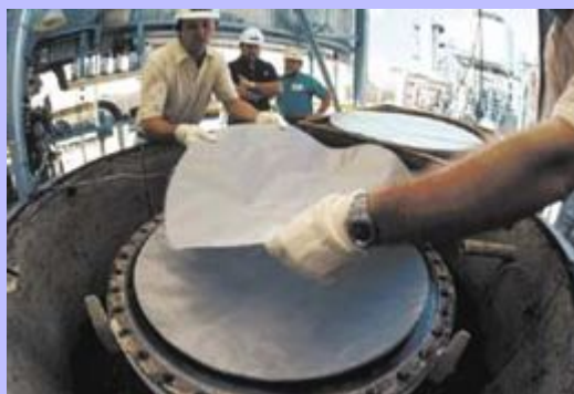
The combustion of ammonia is catalyzed by a gauze of platinum metal.
