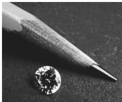
Diamonds and graphite are allotropes of carbon.
