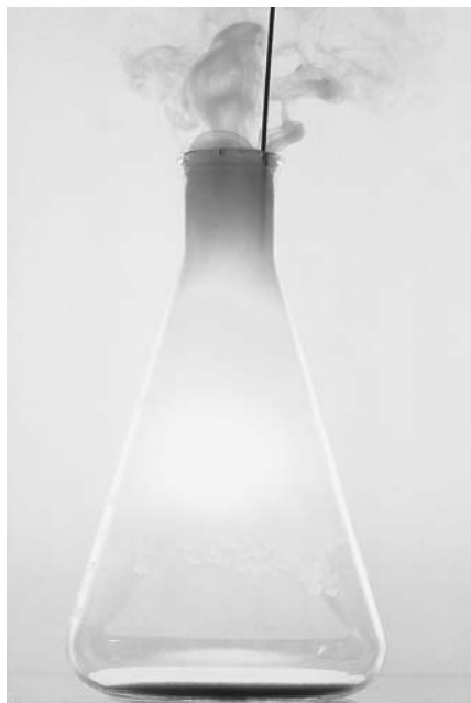
A reaction of sodium with chlorine to produce sodium chloride is an example of a combination reaction.
