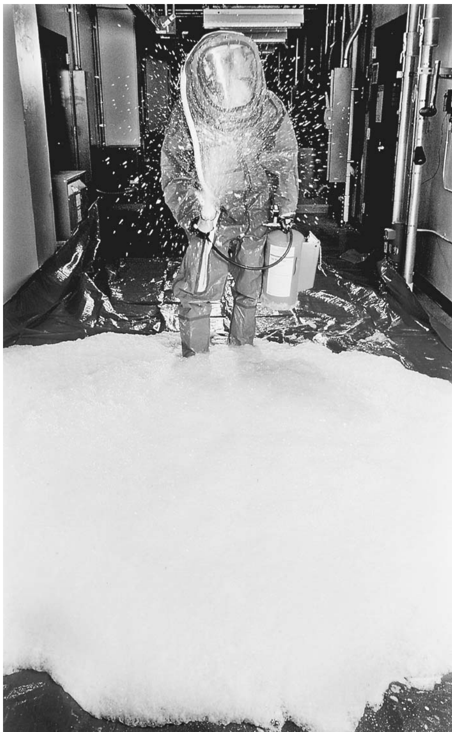
A researcher is spraying decontamination foam in a laboratory to test the neutralization of chemical weapons.
