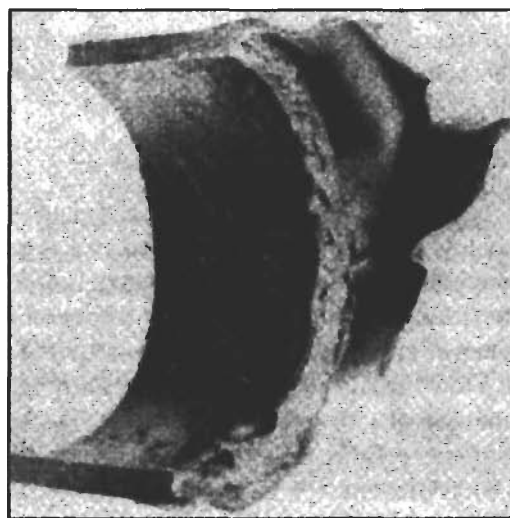
Figure 2. Section of tube at right shows uniform thinning by metal dusting.
