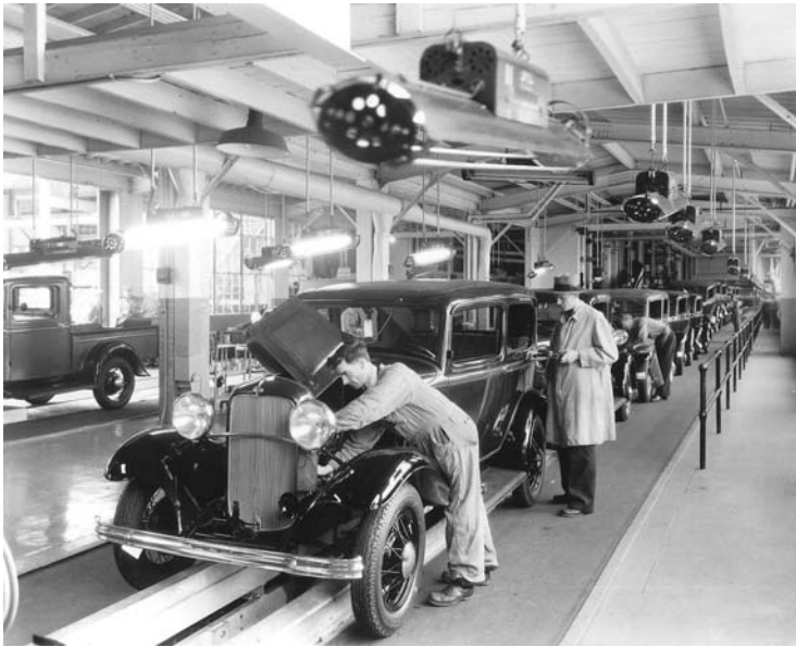
FIGURE 30.1 An early twentieth century Ford assembly line demonstrates the sequential nature of the events that lead to the completed assembly of a series of cars that have gone through the same assembly stages. The auto assembly line is a model for some complex genetic traits. A defect created at any of many steps along the assembly line can result in the same trait—a car whose engine won't run. In theory, a car that fails to turn on and makes no noise when the key is turned could be distinguished from a car in which the engine turns over and then stops. The idea that we can tell the difference between two cars that won't start presumes that we have the ability to distinguish subtleties beyond the fact that this car can't drive away from the factory because the engine doesn't run. Similarly, hits at any of a number of points in a biochemical pathway may cause related traits with the same main characteristics. Such traits might have additional features that can help distinguish the two situations, but if we do not understand enough about the causes of the disease, we may not be able to detect the subtle differences that would let us tell whether we are studying one disease or several different diseases with very different causes but the same final outcome. (Courtesy Detroit News.)
