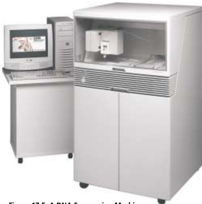
Figure 17.5 A DNA Sequencing Machine Automated DNA sequencing machines can determine DNA sequences rapidly. The machine shown here can sequence a total of over 700,000 bases per day.
