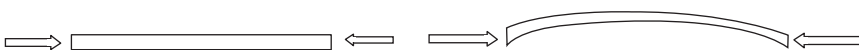
Figure 26.1 A rod that is pressed by two forces is first simply contracting, as in the left figure, but at sufficiently large strain, it buckles out, perpendicular to the forces.
