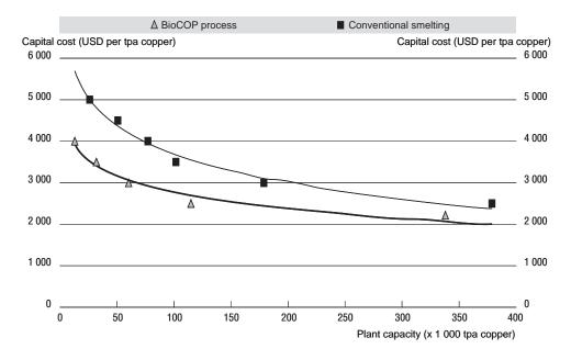
Figure 4. Comparison of capital costs for smelting and bioleaching
