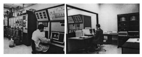
**Fig. 1.** Control of a biotechnological pilot plant in 1978 by a PDP11 computer system. With courtesy of New Brunswick Scientific Co. Inc.
