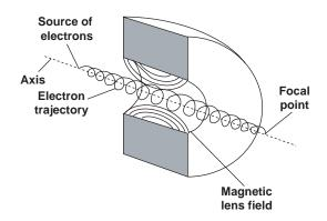
**Figure 4.** Single electron passing through electromagnetic lens. The electron is focused by the magnetic field to follow a trajectory that will converge at a defined focal point after it emerges from the lens.
