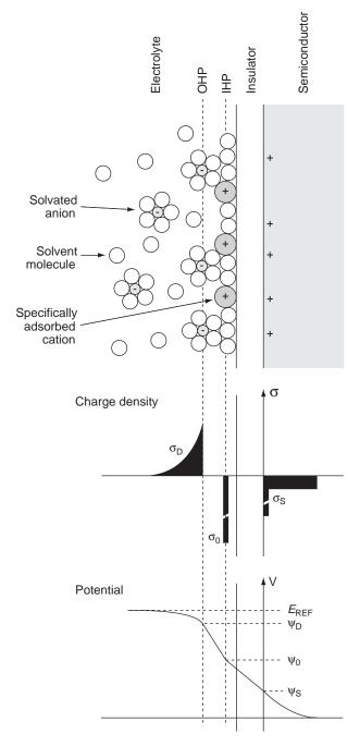
**Figure 3.** Model of the electrolyte-insulator-semiconductor (EIS) system.
