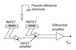
Figure 6. Differential measurement setup for an IMFET.
