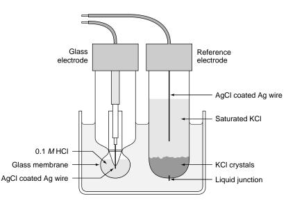
**Figure 1.** Diagram of the glass electrode together with a silver–silver chloride reference electrode.
