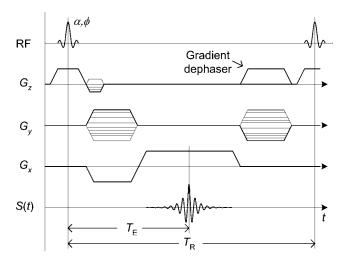
**Figure 8.** Basic 2D gradient echo pulse sequence. First, the magnetization is tipped into the transverse plane by an angle  $\alpha$  during the application of a slice select gradient  $G_z$ . Then, the gradients  $G_y$  and  $G_x$  are used for phase encoding and the readout gradient. An echo forms at  $t = T_E$  when the area under the readout gradient is zero. This experiment is then repeated every  $T_R$  with a different phase encode.
