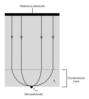
Figure 6. Schematic of two-electrode configuration.
