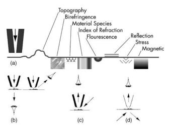
**Figure 4.** Typical apertured NSOM configuration: (a) illustration of information that is carried and can be extracted from the optical signal; (b) transmission and reflection mode NSOM; (c) collection mode NSOM; (d) total internal reflection or dark field mode. (Figure 3b-d adapted from Ref. 17.)
