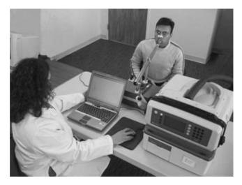
Figure 5. Mensanna portable GC for measuring breath VOCs.
