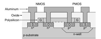
Figure 7. Diagram of the cross-section through a CMOS invertor.
