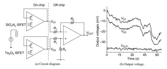
Figure 14. Circuit diagram and graph of output voltage for a differential integrated amplifier based on  $Ta_2O_5$  and  $SiO_xN_y$  ISFETs (15).
