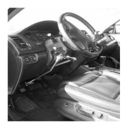
Figure 8. Common hand controls.
