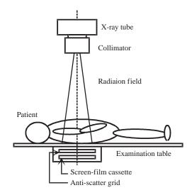
**Figure 1.** Geometric arrangement of conventional radiography. The X-ray system, the anatomy of interest, and the screen-film cassette are centered and aligned for exposure.
