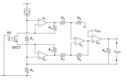
**Figure 12.** Circuit diagram of an ISFET source and drain follower circuit used to maintain a constant drain current at a constant drain-source voltage (42).
