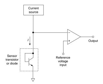
**Figure 1.** A fundamental interfacing circuit of a thermometer making use of a transistor or a diode as a temperature sensor to provide a voltage output proportional to temperature, with a zero voltage output at a specific temperature dependent on the reference voltage selected.
