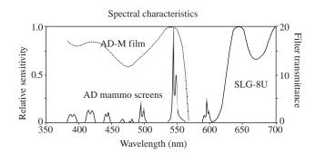
**Figure 5.** Spectral characteristics of screen-film mammography system. The AD Mammo screens are green-emitting and the AD-M film is orthochromatic. The figure shows the light-emitting spectrum of the AD Mammo Screens, the spectral sensitivity curve of the AD-M film, and the transmittance spectrum of SLG-8U safety light filter. (Courtesy of Fujifilm Medical Systems USA, Inc.)
