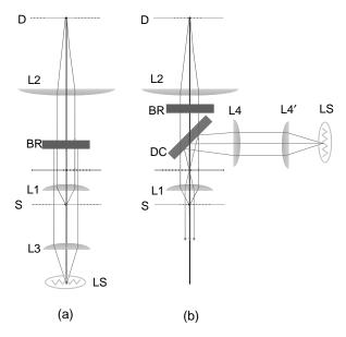
**Figure 4.** Two configurations of fluorescence microscopy (a) trans-illumination and (b) epi-illumination. The objective and detection tube lenses are L1 and L2. The condenser is L3. The excitation relay lenses are L4 and L4'. The sample and detector planes are S and D respectively. The light source is LS. The dichroic filter and the barrier filter are DC and BR.
