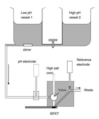
Figure 8. Outline of an Ion-step flow through system.
