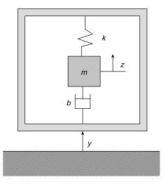
**Figure 4.** Schematic analysis for mechanical movement of a power generator with external vibration.
