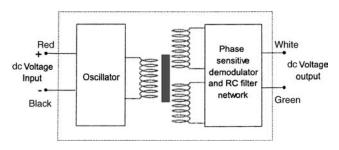
**Figure 4.** Block diagram of a dc LVDT. (Courtesy of Trans-Tek Inc.)
