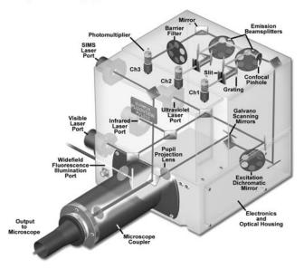
**Figure 3.** Three-channel spectral imaging laser scanning microscope confocal scan head with SIM scanner laser port. The SIM laser enables simultaneous excitation and imaging of the specimen for photobleaching or photoactivation experiments. Also illustrated are ports for a visible, ultraviolet (UV), and infrared (IR) laser, as well as an arc discharge lamp port for widefield observation.
