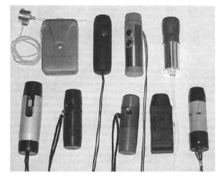
Figure 5. Examples of commercial electrolarynx. (From Ref. 5.)
