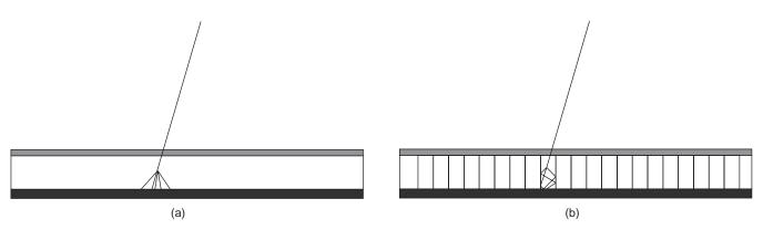
Figure 3. Illustration of EPID conversion screens used to trap optical light. Fig. 3a shows a regular  $Gd_2O_2S$ -screen with optical spread, while Fig. 3b shows a CsI screen which limits optical spread and increases detector resolution.
