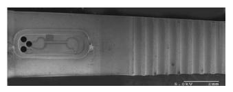
Figure 9. Strain gauges and temperature sensor embedded in robotic microgripper. (Courtesy of Verimetra, Inc.)
