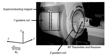
**Figure 1.** Clinical 1.5 T MRI scanner with static field oriented along long axis of the body (z). Patient's head lies in RF coil, which is used to both perturb and receive MR signal. Scanner bed will move patient into middle of cylinder before imaging begins. MR gradient coils for y dimension are shown, which have mirrored coils on the opposite side of the magnet. A portion of the z gradient, based on solenoid design, is also shown.
