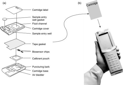
blood samples that have been deposited on a disposable chip. The general procedure for operation is given below (15).
