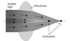
**Figure 5.** Bifocal refractive IOL: Spherical refractive surface that has additional refracting surfaces to give a near add.
