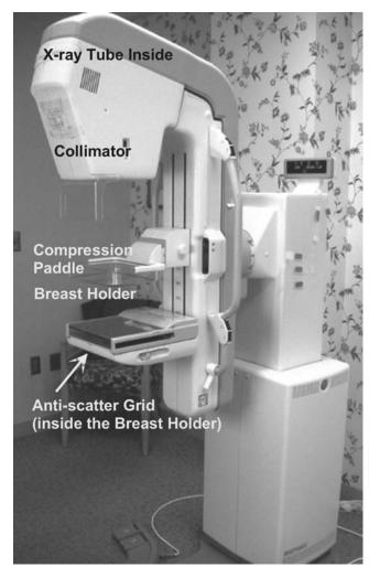
**Figure 4.** A typical dedicated mammography unit; GE Senographe DMR. (Courtesy of GE Healthcare.) The overall mechanical design of a typical dedicated X-ray mammography showing the tilting gantry with the X-ray tube housing at the top and the image receptor at the bottom. The gantry (or the elongated C arm) is normally attached to a column or a stand in which the elevation mechanism of entire gantry is housed.
