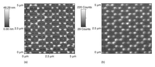
**Figure 9.** Fisher mask, typical structure for NSOM evaluation and calibration: (a) topographic image produced with shear-force feedback; (b) NSOM transmission mode image of the same area. The images were produced on the Aurora-3 NSOM, (Courtesy of Veeco Instruments Inc., Santa Barbara, CA.)
