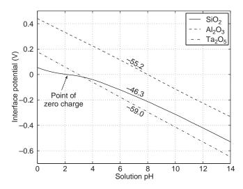
Figure 5. Graph of the theoretical pH response for  $SiO_2$ ,  $Al_2O_3$ , and  $Ta_2O_5$  surfaces.
