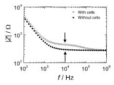
**Figure 13.** Frequency-dependent impedance magnitude for a planar gold-film electrode (d = 2 mm) with and without a confluent monolayer of BAEC directly growing on the electrode surface. The difference in impedance magnitude is maximum at a frequency of 10 kHz.
