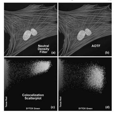
ND Filter versus AOTF Control of Bleedthrough in Confocal Microscopy
