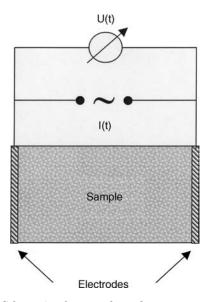
**Figure 1.** Schematic of a two-electrode setup to measure the frequency-dependent impedance of a sample that is sandwiched between two parallel plate electrodes.
