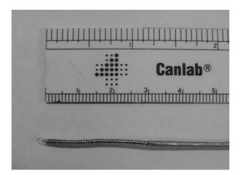
**Figure 4.** Shown here is a BSD Medical (Salt Lake City, UT) helical microwave applicator. The inner conductor of a coaxial cable is extended backward in a helical pattern around the dielectric insulator. There is no connection between the helical section and the outer conductor.
