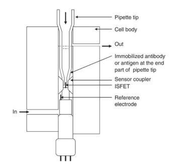
Figure 12. Cross-sectional view of a pH-measuring cell.
