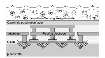
**Figure 8.** Diagram of the cross-section through an ISFET fabricated by an unmodified commercial CMOS process (26). The floating electrode allows the passivation layer to be used as a pH sensitive insulator.
