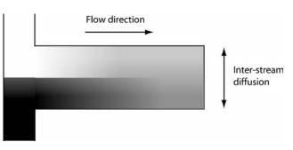
**Figure 4.** Two streams flowing in a microchannel will only mix by diffusion. Note that the concentration across the width of each half of the main microchannel is not constant as diffusional mixing progresses.
