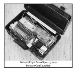
Figure 12. JHU Teeny mass spectrometer.
