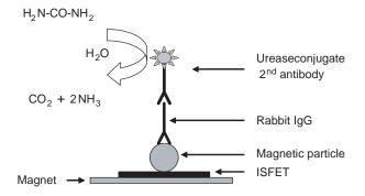
Figure 13. Schematic representation of the magnetoIMFET.
