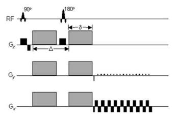
**Figure 11.** Temporal schematic of a diffusion-weighted, spin-echo pulse sequence with an EPI readout. The diffusion gradient pulses are shown as gray boxes on the gradient axes. The direction of diffusion-weighting can be changed by changing the relative weights of the diffusion gradients along  $G_x$ ,  $G_y$ , and  $G_z$ .
