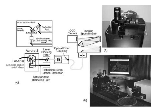
**Figure 8.** Typical, third generation commercially available NSOM setup, for imaging and spectroscopy: (a) photo of the NSOM head and sample holder; (b) complete system with attached spectrometer; (c) optical path schematics. (Courtesy of Veeco Instruments Inc., Santa Barbara, CA.)
