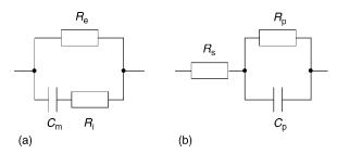
**Figure 1.** RC-networks modeling tissue impedance. The model in (a) mimicks morphological structures, whereas the model in (b) shows the electrically equivalent, but, more usual circuitry.
