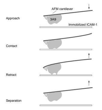
**Figure 7.** Steps in the acquisition of an AFM force measurement. The first step is the approach of the cantilever with a cell bound to the substrate, followed by contact between the cell and substrate and retraction of the cantilever, which results in the separation of the cell from the substrate. The cantilever is bent during this process. The arrows indicate the direction of cantilever movement.
