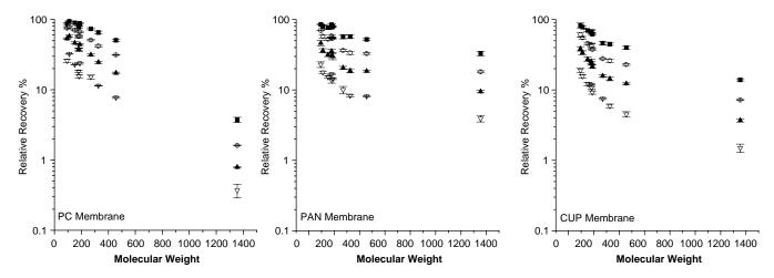
**Figure 2.** Semilog graph of relative recovery versus molecular weight for PC, PAN, and CUP membranes using different perfusion fluid flow rates. Flow rates are  $0.5 \,\mu L \cdot \min^{-1}(\blacksquare)$ ,  $1.0 \,\mu L \cdot \min^{-1}(\bigcirc)$ ,  $2.0 \,\mu L \cdot \min^{-1}(\blacktriangle)$  and  $5.0 \,\mu L \cdot \min^{-1}(\blacktriangle)$ . Adapted from Ref. 29).
