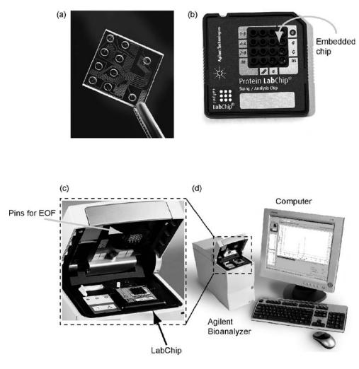
Figure 9. (a) The Bioanalyzer uses microfluidic chips etched from glass. (Images courtesy of Agilent Technologies). (b) The etched glass chips are encased in a plastic assembly that facilitates handling and limits contamination. Images courtesy of Agilent Technologies. (c) Samples are loaded onto the chip and the chip is loaded into the Bioanalyzer. (Images courtesy of Agilent Technologies). (d) The Bioanalyzer then performs an analysis on the samples. (Images courtesy of Agilent Technologies.)
