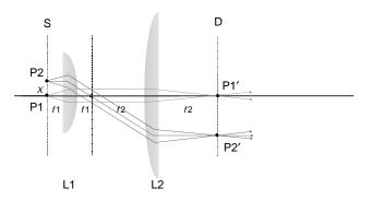
**Figure 3.** The detection path of a microscope. Lenses L1 and L2 are the objective and the tube lens, respectively. L1 has focal length f1 and L2 has focal length f2. For two points, P1 and P2 with separation, x, on the sample plane (S), these points are projected to points P1' and P2' on the detector plane (D).
