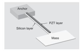
Figure 6. Structure of a piezoelectric cantilever for power generation.
