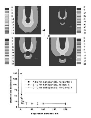
**Figure 6.** Finite-element methods (FEM) simulation of the electromagnetic field scattering and near field enhancement at the apex of the tip of the apertureless NSOM, and its behavior with change in tip-sample separation distance. (Adapted from Ref. 30.)
