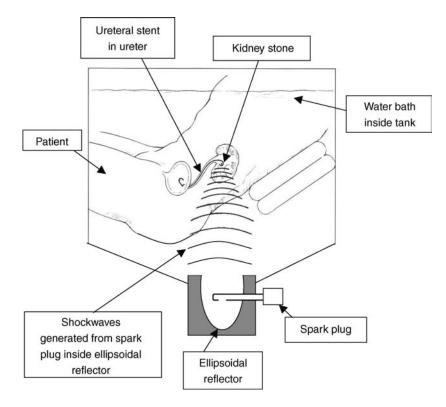
**Figure 1.** Schematic diagram of noninvasive extra corporeal shockwave lithotripsy (ESWL) procedure used to disintegrate kidney or biliary stones. Acoustic waves generated from spark plugs are focused with ellipsoidal reflectors on the kidney stone.
