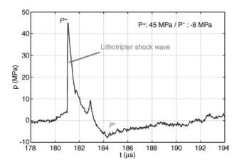
**Figure 1.** Pressure–time relationship of typical shock waves. Typical pattern of a lithotripter-generated shock wave. The shock wave is characterized by a leading positive or compressive component (P+) followed by a negative or tensile component (P-).
