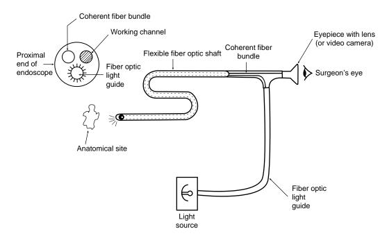
Figure 2. Components of a typical endoscope.
