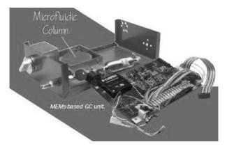
Figure 7. LLNL MEMS-based micro-GC.
