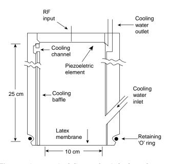
**Figure 6.** A cross-sectional diagram of a single planar element hyperthermia applicator. The chamber between the latex membrane and the piezoelectric element contains cooled degassed water. During local hyperthermia treatment an ultrasonic conducing gel is applied to the target site that is then coupled to the latex membrane. (Published with permission from Ref. 3).
