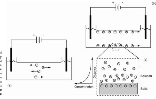
**Figure 5.** (a) Electrophoresis. Charged particles will move toward oppositely charged poles in an elec- tric field. (b) Electroosmosis. Charges lining a microchannel sur- face will move with an applied electric field, thus inducing bulk flow via momentum transfer within the liquid. (c) An electric double layer forms at charged microchannel surfaces; the layer thickness is called the Debye length.
