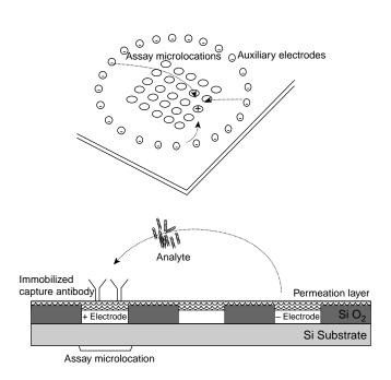
**Figure 7.** Active electronic microchip technology. (a) Basic chip layout; (b) Cross-section of microchip for electrophoresis of proteins (29).
