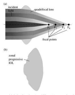
**Figure 6.** Multifocal refractive IOLs: (a) several refractive surfaces with different curvatures. Each one provides a focal point (b) a commercial zonal progressive IOL with five concentric zones on the anterior surface. Each zone repeats the entire refractive sequence corresponding to distance, intermediate and near vision, resulting in wide-range vision.
