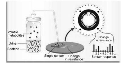
Figure 8. Osmetch Microbial Analyzer detection technology (31).
