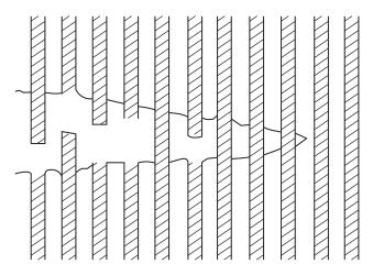
**Figure 10.** Model of crack tip in a fiber-reinforced composite showing how a crack may propagate Fibers become debonded from the matrix and are pulled out as the crack widens.
