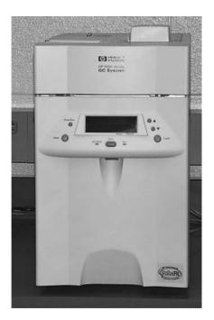
Figure 4. An HP/Agilent laboratory-grade gas chromatograph.
