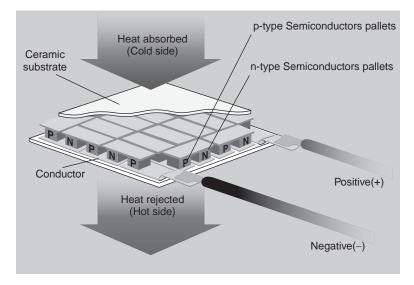
**Figure 2.** Principles of thermoelectric power source (Biophan).
