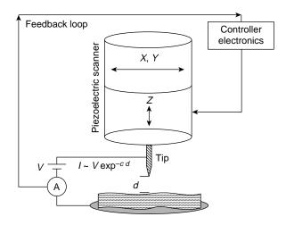
Figure 6. Important features of an STM system.
