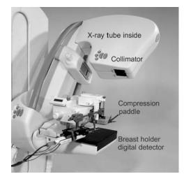
**Figure 12.** Photograph of GE FFDM unit; Senographe DS with stereotactic attachment installed. The gantry is tilted to  $+15^{\circ}$  and prepped for Stereotactic imaging. Note, this is the FFDM version of similar unit shown in Fig. 1, but with zoomed up view for the stereotactic attachment. (Courtesy of GE Healthcare.)
