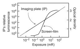
**Figure 7.** Comparison of dynamic range of CR and screen-film image receptors. (Courtesy of Fuzifilm Medical Systems, USA, Inc.) The image plate (IP) has wider linear response to radiation extends over four decades of dose and eliminates the inherent limitations of the "toe" and "shoulder" portions of the film's H&D Curve. (Courtesy of Fujifilm Medical Systems USA, Inc.)
