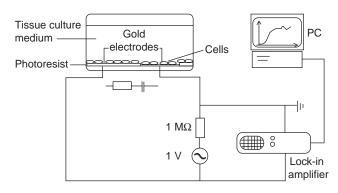
Figure 7. The ECIS measurement setup.
