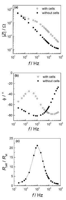
**Figure 9.** (a, b) Bode-diagrams of an ECIS electrode with confluent MDCK cells and an empty electrode. (c) Plot showing the division of the measured resistance of an ECIS electrode with confluent MDCK cells with the corresponding values of the empty electrode plotted versus log f.
