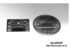
**Figure 13.** MEMS TOF mass spectrometers developed at Ajou University in Korea.
