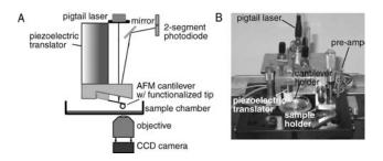
**Figure 6.** AFM experimental set-up. (a) Schematic diagram of the AFM. (b) Photograph of the author's AFM setup. The CCD camera is not in view.
