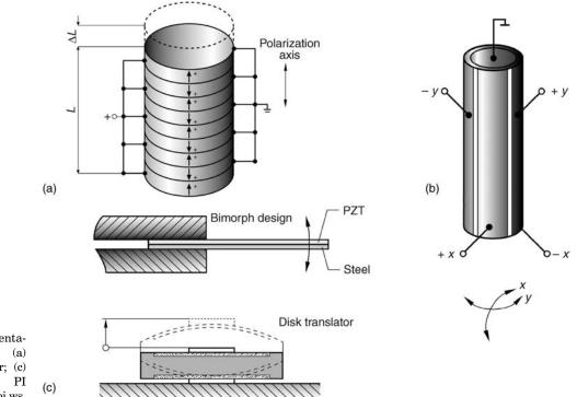
Figure 2. Schematics representation of the piezo actuators: (a) stacked piezo; (b) tube scanner; (c) bimorph scanner. [Courtesy PI (Physik Instru-mente) LP, www.pi.ws.
