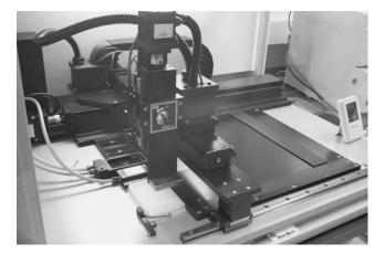
Figure 4. A microarraying robot. The robotic arrayer prints DNA onto glass slides with very high precision. Robots such as this have extremely high accuracy, on the order of 10  $\mu$ m or less.
