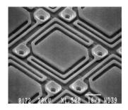
Figure 14. 25 micron wide longwave IR microbolometer detector.
