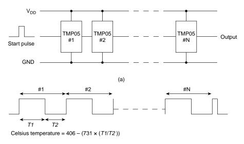
Figure 6. (a) The connecting scheme for a daisy chain operation of a serial-digitaloutput-type temperature sensor, and (b) the output waveform. The temperature using the Celsius scale at each sensor can be determined from the ratio of the duration of the highest and lowest points in each cycle.
