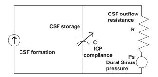
**Figure 2.** Electric circuit analog model of CSF system. In this model, current represents flow of CSF fluid, and voltage represents pressure. The capacitance C, represents intracranial compliance, and the resistance R represents resistance of CSF fluid flow into the venous system.
