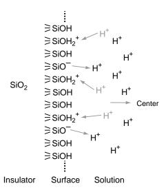
**Figure 4.** Diagram illustrating the surface sites and hydrogenion reactions for  $SiO_2$ .
