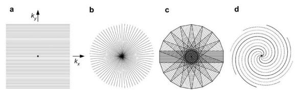
**Figure 9.** 2D k space sampling trajectories. Shown are the spin-warp (a), radial sampling (b), PROPELLER (c), and interleaved spiral imaging (d) examples.
