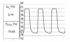
Figure 10. Oxigraf Fast Oxygen Sensor trace of respired O<sub>2</sub>.
