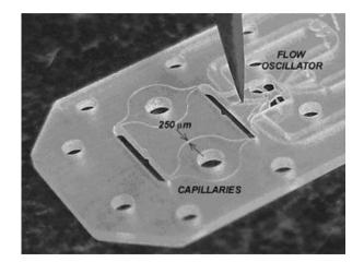
Figure 15. Microfluidic chip that measures the density and viscosity of three-component respired gases from which the constituent gas concentrations of oxygen, nitrogen, and carbon dioxide are deduced.
