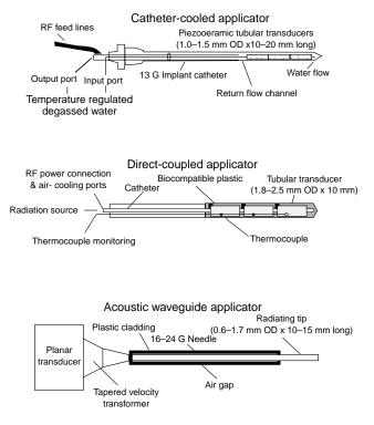
**Figure 16.** Interstitial hyperthermia catheters. (Published with permission from Ref. 7).
