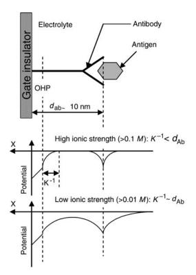
**Figure 4.** Schematic representation of the potential distribution in a direct-acting IMFET.  $K^{-1}$  is the Debye length;  $d_{Ab}$ , dimension of macromolecule (e.g., antibody).
