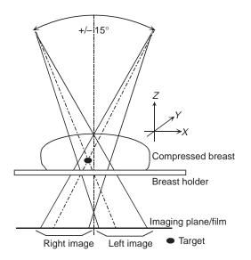
**Figure 8.** Schematic drawing of geometrical setup for stereotactic mammography. From the stereo images, with known geometry and the X-Y coordinates, the depth in Z direction is calculated via triangulation.
