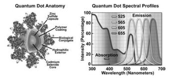
**Figure 15.** Anatomy and spectral profiles of quantum dot conjugates. The cadmium selenide core is encapsulated with zinc sulfide, and then a polymer coating is applied followed by a hydrophilic exterior to which the biological conjugate is attached (left). The absorption profile displays a shoulder at 400 nm, while the emission spectra all feature similar symmetrical profiles.
