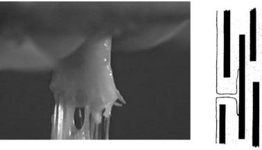
Figure 3. (a) Video image showing a ligament failing under tensile strain. (b) A schematic diagram showing a longitudinal section through a fiber composite illustrating how a weak matrix prevents crack propagation from one fiber to another and dissipates its energy by creating cracks in directions other than across the composite.
