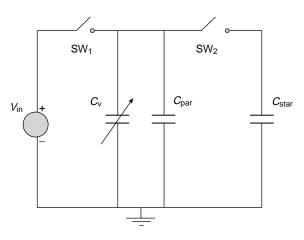
**Figure 7.** Circuit representation for an electrostatic converter (15).
