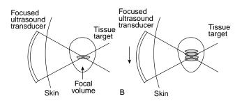
**Figure 17.** Schematic of HIFU. (a) Illustrates a formation of a single lesion. (b) Illustrates a confluent array of lesions required for a therapeutic effect. (Published with permission from Ref. 98).
