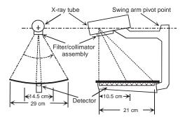
**Figure 13.** A schematic drawing of the scanning mechanism of Fischer Senoscan FFDM. (Adapted from Fisher Imaging Sanoscan user's manual with permission. Courtesy of Fischer Imaging.)
