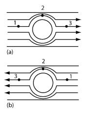
**Figure 2.** (a) A suspended particle in laminar flow around an obstacle in a microchannel. (b) If the flow is reversed, the particle will retrace the same path.
