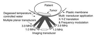
**Figure 14.** A schematic diagram of mechanically scanned ultrasound system for superficial hyperthermia. (Published with permission from Ref. 7).
