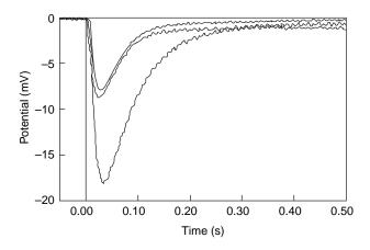
**Figure 9.** Ion-step responses of HSA-coated ISFET before (upper solid curve) and after incubation (for 15 min) with undiluted anti-HSA (lower solid curve) and anti-BSA (dashed curve). Ion stepping was performed at pH 4.02.
