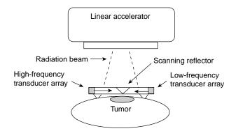
Figure 13. A schematic diagram of a multielement low profile scanning reflector system. (Published with permission from Ref. 7).
