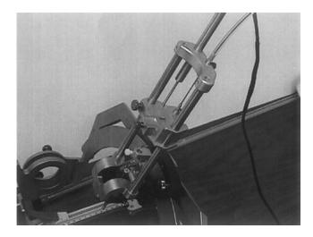
**Figure 6.** Mechanism of modular brain probe drive showing the LVDT used to help in precise electrode placement. [Courtesy of Radionics (a division of Tyco Healthcare).]
