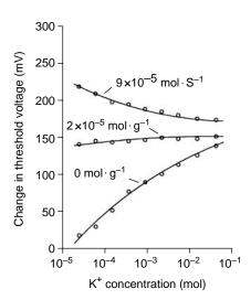
**Figure 18.** Graphs of the response of an acrylate REFET, and an ISFET, to changes in potassium and hydrogen ion concentrations (53).
