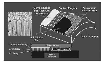
**Figure 11.** Schematic drawing of an amorphous silicon digital detector. (Courtesy of GE Healthcare.)
