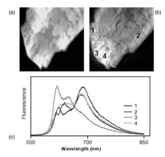
**Figure 7.** Example of fluorescence-based hyperspectral near-field imaging. (a) Shear-force topography image; (b) NSOM fluorescence image; (c) spatially resolved fluorescence spectra, numbers 1–4 corresponds to the different position on the crystal, demonstrating chemically specific imaging and material inhomogenities at the nanoscale. (Courtesy of David Vanden Bout and Paul Barbara, University of Minnesota, Minneapolis, MI.)
