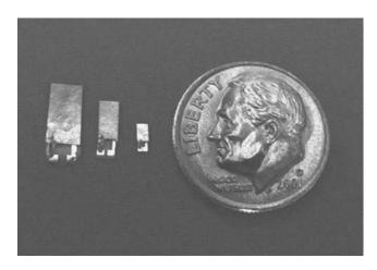
**Figure 11.** Ultrasound transducers next to a dime. (Courtesy of Verimetra, Inc.)
