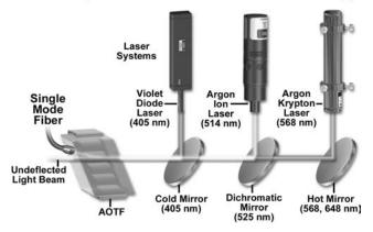
Figure 9. Configuration scheme utilizing an AOTF for laser intensity control and wavelength selection in confocal microscopy.
