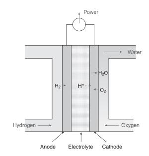
Figure 1. Schematic of a PEM fuel cell.
