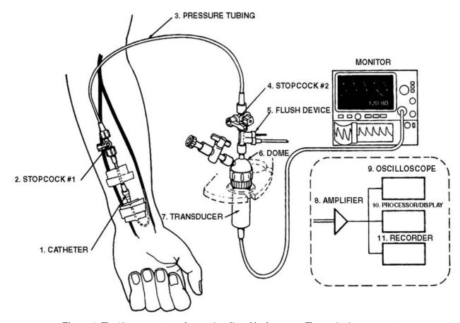
**Figure 4.** The 10 components used to monitor direct blood pressure. The monitoring components are nearly independent of whether the catheter is in an artery (radial, brachial, or femoral) or in the pulmonary artery. Size of transducer and plumbing components are enlarged for illustration purposes. [Reproduced from Ref. 6, with permission.]
