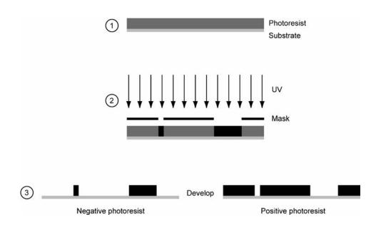
Figure 8. Photolithography requires an ultraviolet (UV) light source, a mask, and a photosensitive layer of material (i.e., photoresist). The photoresist is patterned with the UV light via a mask.
