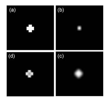
**Figure 14.** Clockwise from upper left: (a) synthetic true image (b) Gaussian PRF, (c) degraded measurement, and (d) restored image.
