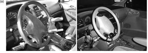
Figure 7. Steering knobs.
