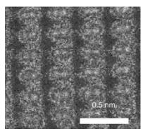
**Figure 1.** Image of a silicone crystal observed in the [112] orientation recorded with an aberration corrected STEM. (From Ref. 1). Reproduced by courtesy of American Association for the Advancement of Science.)
