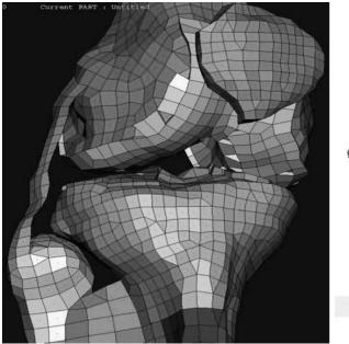
**Figure 13.** (a) Knee FE model components shown in different color-implicit formulation (102) (b) the knee FE model during simulation of single leg-hopping-explicit formulation (103).
