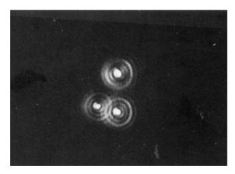
**Figure 3.** Airy disks generated by viewing three pinholes in a light microscope. Magnification of micrograph is  $1000 \times$ . (From Ref. 4. Reproduced by courtesy of Jones and Bartlett Publishers.)
