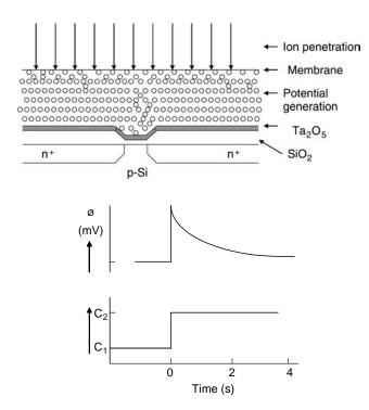
**Figure 5.** An ion-step arrangement: an ISFET exposed to an increased electrolyte concentration. Transient potential can be measured, developing from transient transport of ions across the membrane, which is caused by stepwise changes in electrolyte concentration. The ISFET response  $\phi$  as a result of the stepwise changes in electrolyte concentration ( $C_1$ - $C_2$ ).
