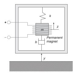
Figure 5. Schematic of an electromagnetic conversion device.
