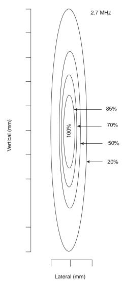
**Figure 5.** The intensity distribution in the focus of an ultrasound transducer. The diameter and the length are a function of frequency. The lower the frequency, the larger the diameter, and the smaller the aperture, the longer the focal region. (Published with permission from Ref. 3).
