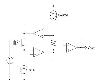
Figure 13. Circuit diagram of constant drain current, constant drain-source voltage ISFET bias circuit (43).
