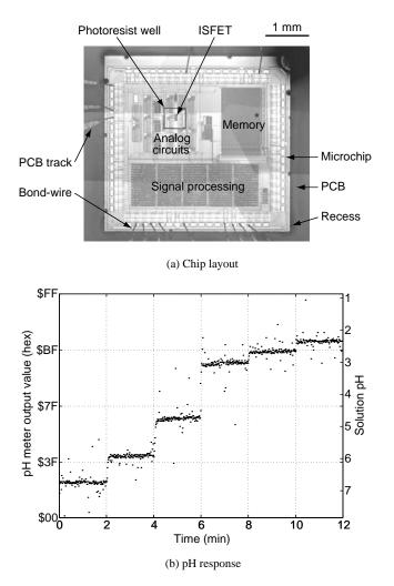
**Figure 15.** Chip layout and pH response of a single-chip digital pH meter.
