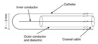
**Figure 3.** A schematic representation of a microwave interstitial dipole antenna applicator. The outer conductor of a coaxial cable is stripped away to produce a radiating section.
