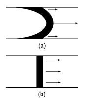
**Figure 6.** (a) Pressure-driven flow is parabolic; the middle of the stream moves faster than regions near the wall. (b) Electrokinetic flow is blunt; all parts of the stream move at equal velocity. Note that residual pressures can cause the profile to become slightly parabolic in the direction of the negative pressure gradient.
