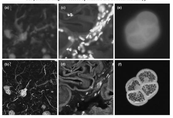
Comparison of Images Produced by Widefield and Confocal Microscopy
