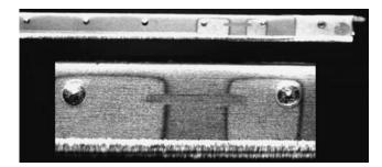
**Figure 8.** Strain gauges fabricated on surgical sharps. (Courtesy of Verimetra, Inc.)
