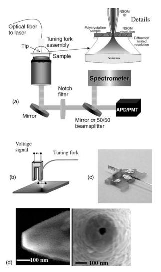
Figure 3. Example of the aperture-based, straight-fiber NSOM: (a) schematics representation of the scanning probe and collection; (b) schematics representation of the tapered fiber NSOM probe, attached to the tuning fork; (c) photography of the probe glued to the tuning fork; (d) SEM image of the end of the tapered, aluminum-coated fiber optic based NSOM probe. (Courtesy of Veeco Instruments Inc., Santa Barbara, CA.)
