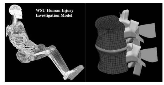
Figure 16. The Wayne State University full body impact model and the spine model (130,135).
