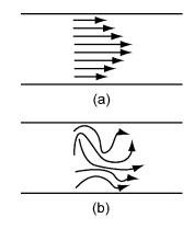
**Figure 1.** (a) Particles suspended in a laminar flow within a straight microchannel follow straight trajectories. (b) Particles suspended in a turbulent flow within a straight microchannel do not follow straight trajectories unless they are very close to the wall.
