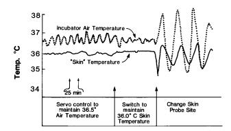
**Figure 7.** Example of variations in dynamic air temperature changes when an enclosed incubator that was initially servo controlled to maintain a stable air temperature was switched to a skin temperature referenced servo control mode and then was perturbated by changing the site of attachment of the skin temperature-sensing thermistor. The wide thermal cycling illustrated as a consequence of this sequence continued for 3 h before returning to a more stable pattern.
