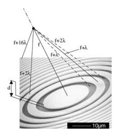
**Figure 3.** Binary diffractive phase element: Fresnel zone plate. Waves traveling along various segments arrive in phase at the focal point since the optical paths differ by a multiple of the wavelength. To fulfill this condition, the thickness *d* is chosen so that it introduces a phase shift of  $\pi$ :  $d = (2k + 1) \lambda/[2(n-1)]$  (optical path:  $(2k + 1) \lambda/2$ ): In the figure, k = 0.
