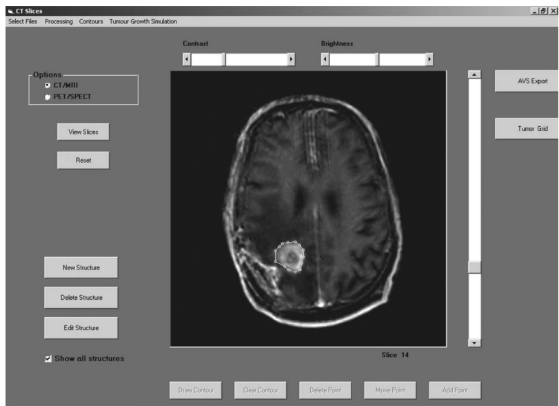
FIGURE 5.1. The interface of the dedicated software tool for the delineation of anatomical structures of interest and the preprocessing procedure of the imaging data.
