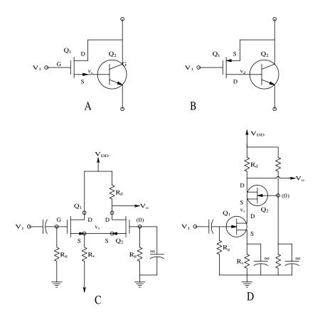
(A) An n-channel MOSFET/npn BJT Darlington configuration. (B) A p-channel MOSFET/npn BJT feedback pair configuration. (C) An n-channel MOSFET source-follower–grounded-gate amplifier. (D) An n-channel JFET cascode amplifier.
