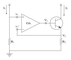
4.7 The op amp circuit shown in Figure P4.7 is a form of current mirror. The BJT can be modeled by its MFSSM with  $h_{re} = h_{oe} = 0$ . The op amp is ideal except for the gain:
